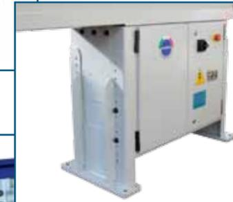
The mechanical syncro device ties the barfeeder rigidly to the lathe regardless of the headstock speed or the bar thinness.
