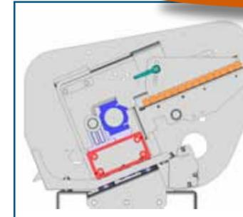
The new Boss HD (Heavy Duty) structure guarantees the barfeeder absorbs a larger quantity of vibration from the rotating bar (even over 60%) shielding the lathe headstock.
